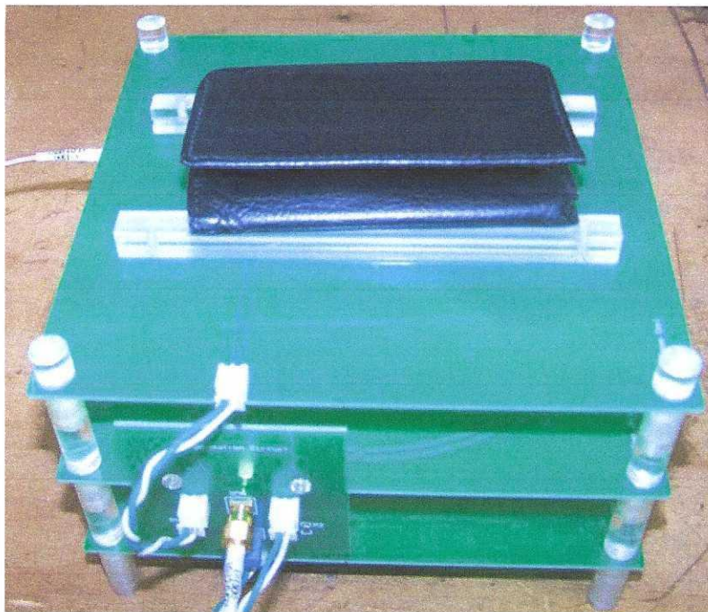
Figure 14 – Wallet placed in front of RFID Scanner
